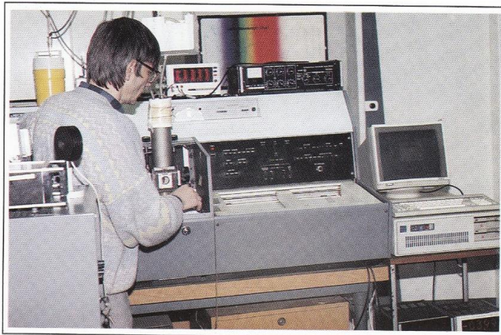
M. Sc. M. Kaczmarek at the apparatus for Raman scattering investigation.
