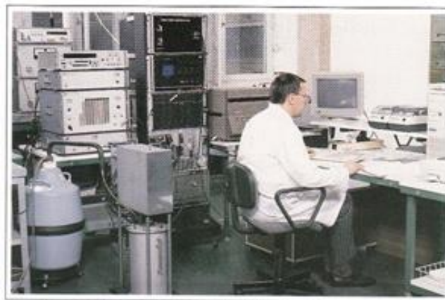
The complete commercial version of the FT NQR spectrometer, operating in the frequency 0.5-300 MHz and developed in cooperation with MBC ELECTRONICS, Warsaw.
