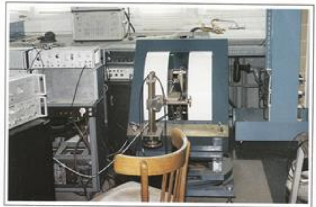
Spectrometer for measurements of selfdiffusion coefficients by NMR technique.
