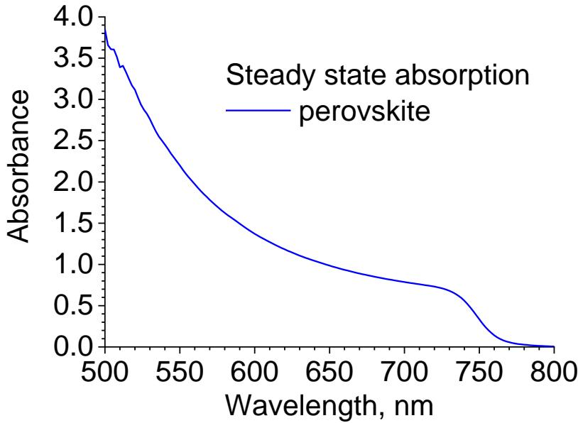
In the typical samples more than 80% of light is absorbed within the first 100 nm of perovskite layer for the excitation wavelength below 500 nm.
