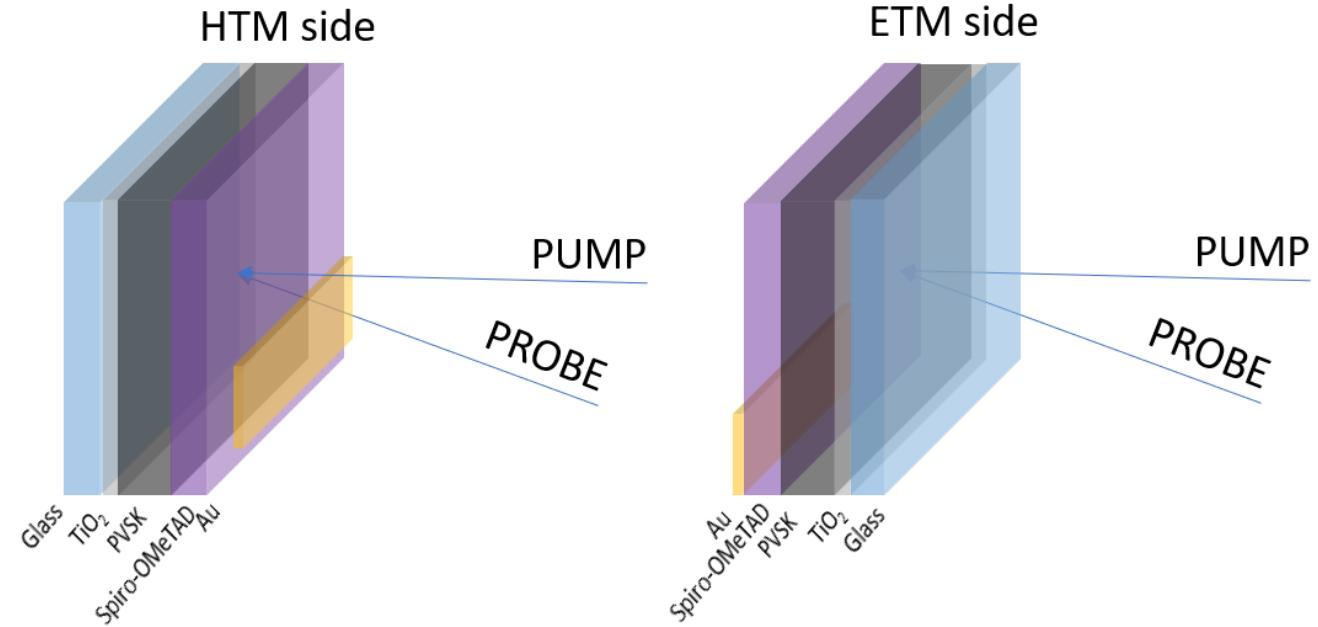
Transient absorption can be used as very unique interface selective steady-state probing!
