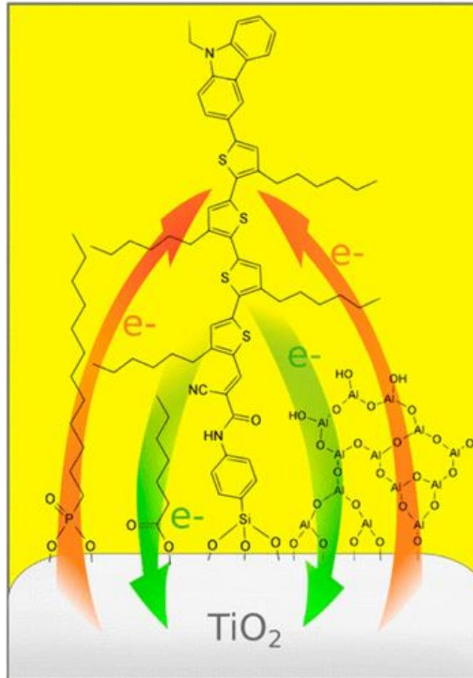
Determination of charge injection and recombination in transient absorption:
