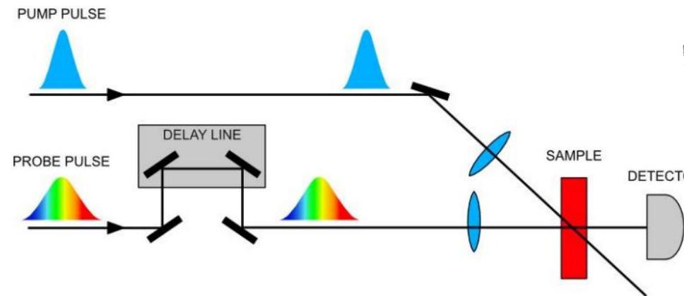
We need laser pulses to measure very short charge transport times in solar cells.
